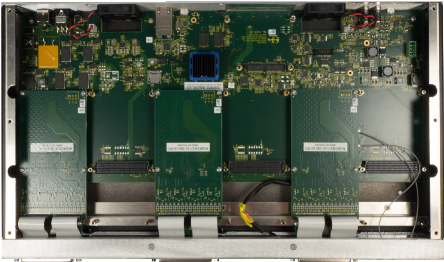
Figure 4: Example Fitted to ACQ2106 Carrier, 96 channels in 1U
